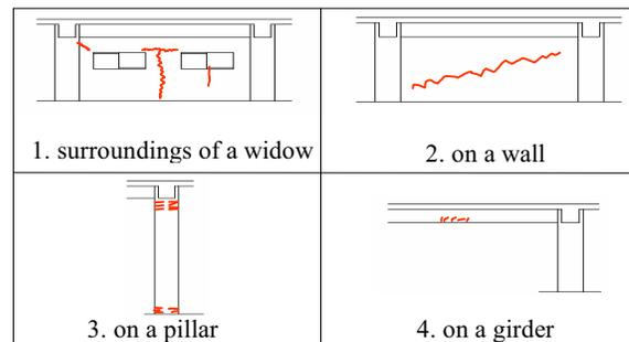
Figure 1. The place where cracks occur
