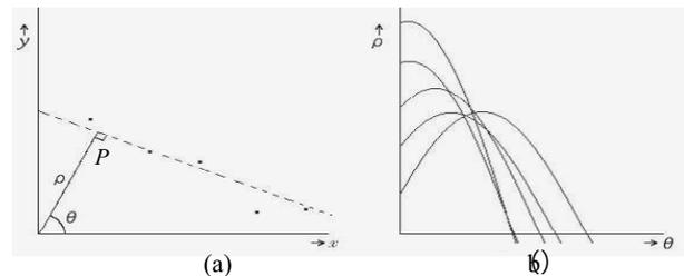
Figure 4. Hough conversion; (a) edge points of  $x$ - $y$  space (b) locus of  $\rho$ - $\theta$  space
