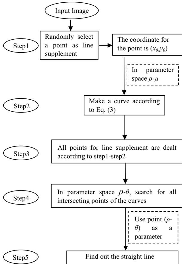
Figure 6. Hough conversion Algorithm
