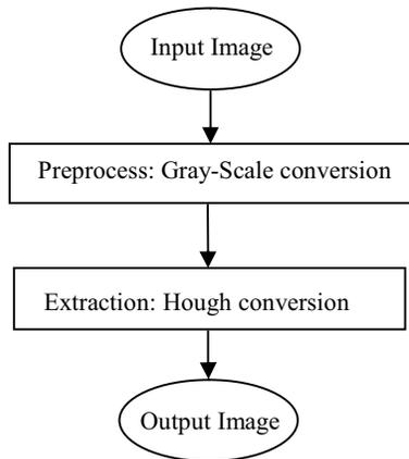
Figure 3. Flowchart of cracks extraction with image processing technology
