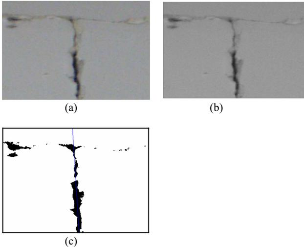
Figure 9 . Cracks in a crisscross pattern in the beams; (a) original image (b) grayscale (c) Hough
