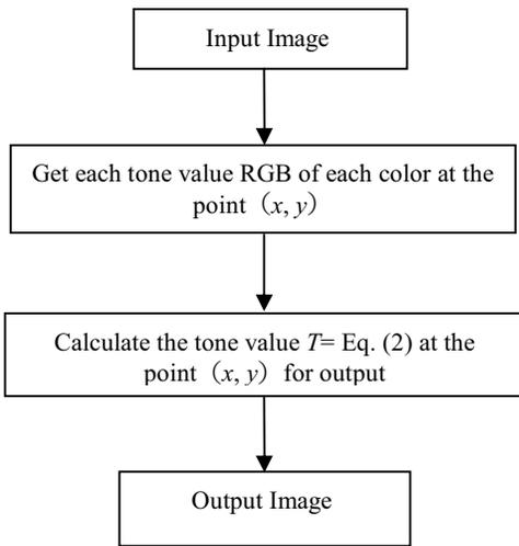
Figure 5. Grayscale conversion algorithm
