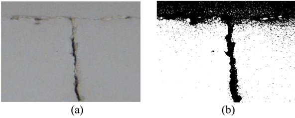
Figure 2. Binarization without preprocessing; (a) original image (b) binarized image
