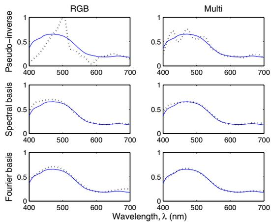
Figure 2. Reconstructed (dashed lines) and measured (full lines) spectral reflectance, using model-based characterization.
