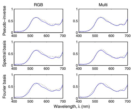
Figure 3. Reconstructed (dashed lines) and measured (full lines) spectral reflectance, using empirical characterization.
