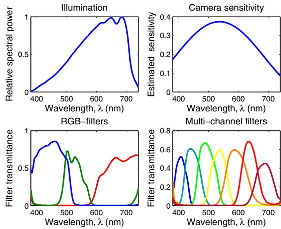
Figure 1. Spectral power for the illuminant (a), estimated spectral sensitivity for the camera (b) and spectral transmittance for the RGB filters (c) and the 7 multi-channel filters (d).
