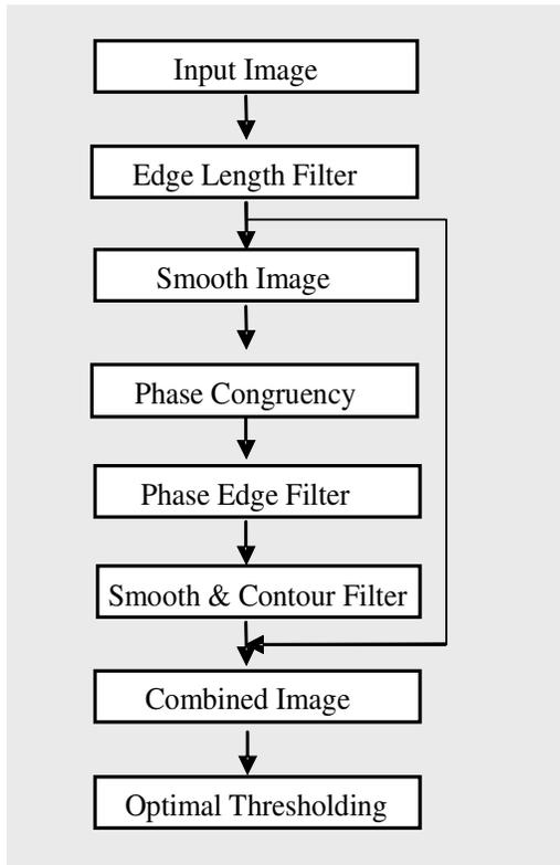
Fig. 4. Block diagram of the proposed algorithm.
