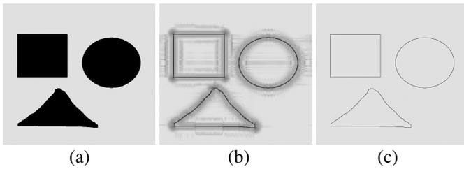
Fig. 3. (a). Original image. (b) Phase congruency image (c) After apply edge filter
