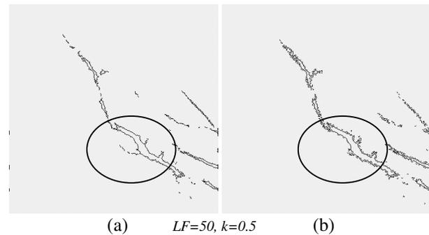
Fig.5 (a) Contour based image segmentation using phase congruency for edge detection. (b) Contour based image segmentation using Canny method for edge detection.
