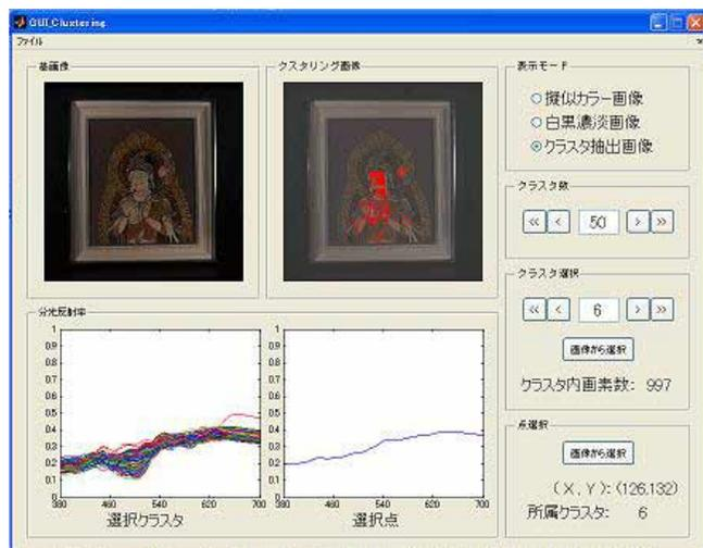
Figure 7. GUI-based segmentation tool developed.
