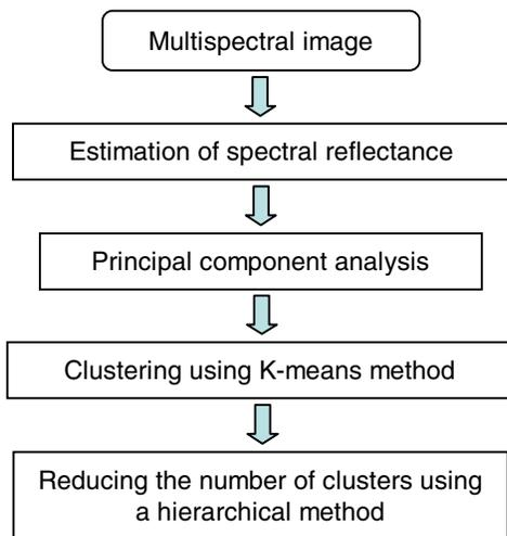
Figure 6. Processing flow for multispectral image based clustering.
