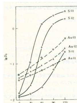
Fig.1 The dependence of fog formation on sensitizing time in developer D-19b.
