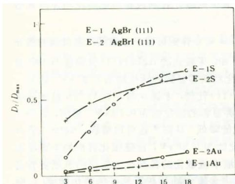
Fig.3 The dependence of fog formation on developing time in developer D-19b at 20°C
