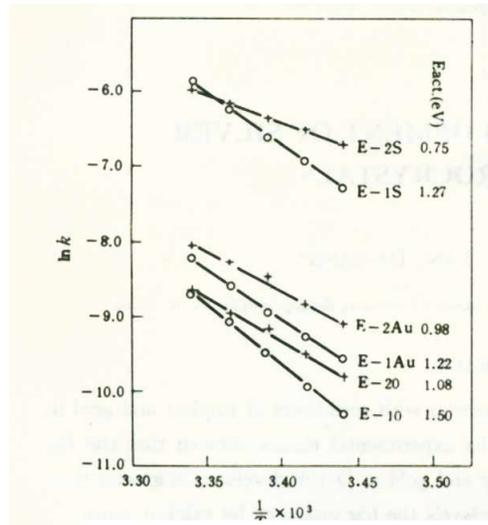
Fig.5 Arrhenius plot of fog formation for different sensitizer added in developer D-19b, E-10, E-20 unsensitized emulsion.
