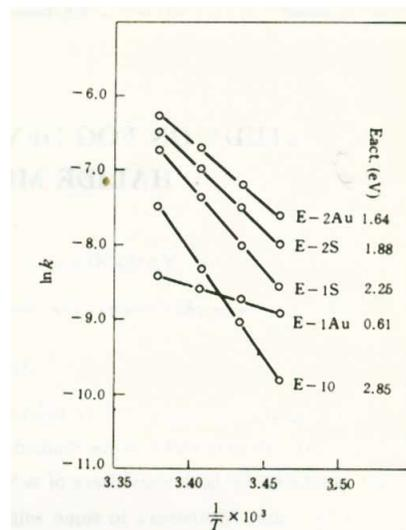
Fig. 6 Arrhenius plot of fog formation for different sensitizer added in developer CD-4, E-10 unsensitized emulsion.
