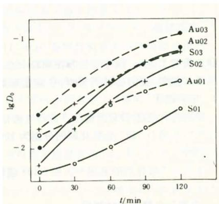
Fig.2 The dependence of fog formation on sensitizing time in developer CD-4.
