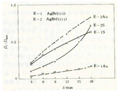
Fig.4 The dependence of fog formation on sensitizing time in developer CD-4 at 20°C.
