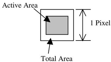
Figure 1. Pixel schematic
