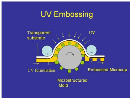
**Figure 1:** UV forming process for lens manufacture [2]
