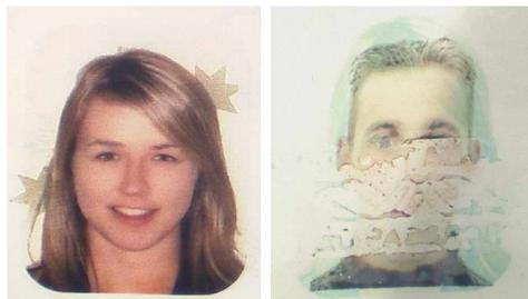
**Figure 5:** Inkjet printed data before tampering (left) and after tampering and overprinting (right)
