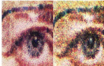
**Figure 4:** Inkjet print comparison between intelligent coating (left) and paper (right) – (x40 magnification)
