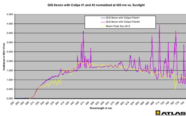
Figure 1. Comparison of spectral power distribution of natural sunlight and filtered xenon.
