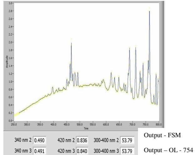
**Figure 3.** Comparison of conventional spectroradiometer output with FSM system
