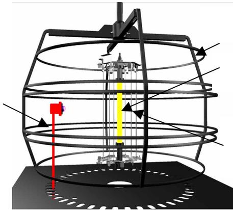
**Figure 2.** Graphical display of the lightfastness chamber interior. CCD array spectroradiometer is mounted below the test chamber.
