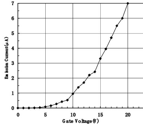
Figure 3 I-V characteristics of the Gated Transfer Mold Mo FEAs
