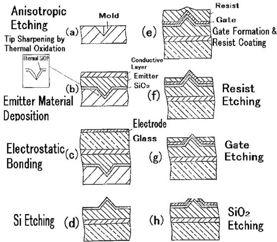
Figure 1 Transfer Mold fabrication process
