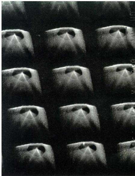
Figure 2 SEM micrograph of the Gated Transfer Mold Mo FEA
