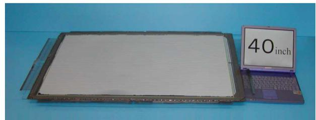
Figure 4 triode type 40-inch size CNT-FED
