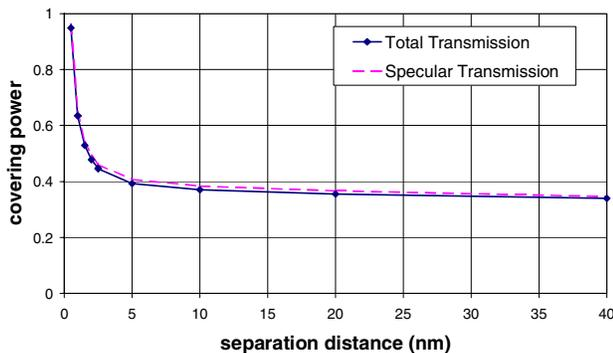
**Figure 3.** Calculated covering power for randomly oriented  $3 \times 3 \times 3$  cubic clusters of twenty-seven 10-nm-diameter silver spheres in a 20- $\mu\text{m}$  layer with a silver loading of 1.9  $\text{g}/\text{m}^2$ .
