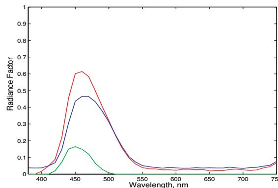
Figure 4. Radiance factor of Golden Acrylic Blue; the red, blue, and green lines are total, reflectance, and luminescence radiance factors, respectively.
