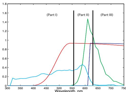
Figure 1. Emission (green line) and excitation (cyan line) spectra of Golden Acrylic Orange along with the optimized excitation filters; the red line is transmittance of the fluorescence-weakening filter, and the blue line is transmittance of fluorescence-killing filter.
