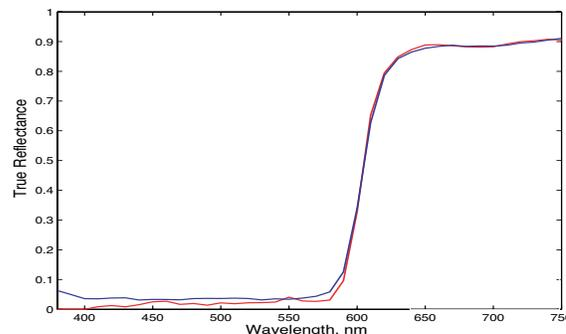
Figure 3. True reflectance of Golden Acrylic Orange; the blue line is measured with the Labsphere 450 bispectrometer and the red line is reconstructed using Allen's method.
