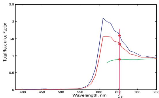
Figure 2. Total radiance factor of Golden Acrylic Orange with and without excitation filters; the blue line is without the filter, the red line is with the fluorescence-weakening filter, and the green line is with the fluorescence-killing filter.
