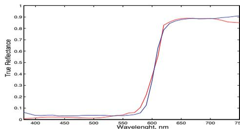
Figure 6. True reflectance of Golden Acrylic Orange; the blue line is measured with the Labsphere 450 bispectrometer and the red line is reconstructed using abridged fluorescence imaging.
