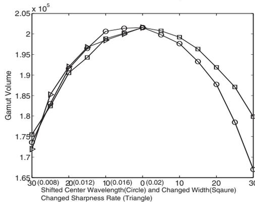
Figure 7. The effects of shifting center wavelength (circle), changing width (square), and changing sharpness rate (triangle) of magenta ink on color constancy.
