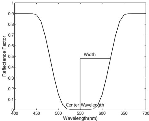
Figure 1. The ink spectral reflectance curve produced by the trapezium function with two peak wavelengths. The sharpness rate  $k$  was set to  $-0.02$ , the peak wavelength to  $550\text{nm}$ , and the bandwidth to  $60$ .
