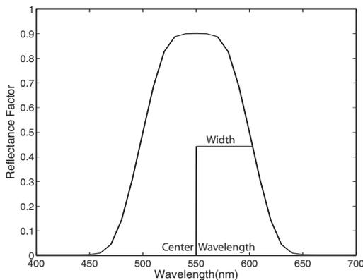
Figure 2. The ink spectral reflectance curve produced by the trapezium function with a single peak wavelength. The sharpness rate  $k$  was set to  $0.02$ , the peak wavelength to  $550\text{nm}$ , and the bandwidth to  $60$ .
