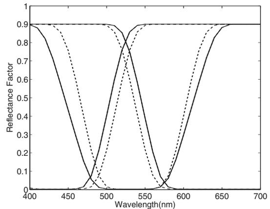
Figure 6. Spectral reflectance factor comparison between the three-ink set optimized for maximum gamut volume (dashed line) and minimum color inconstancy (solid line) with a 5% gamut volume compromise.
