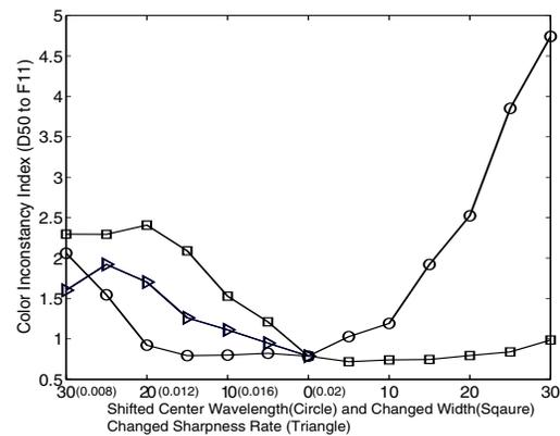
Figure 8. The effects of shifting center wavelength (circle), changing width (square), and changing sharpness rate (triangle) of magenta ink to the color constancy.
