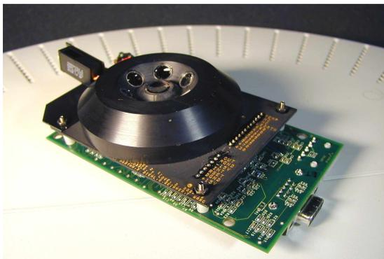
**Figure 3:** Photograph of LCLEDS Sensor Head from the Top Showing Details of the Lenses, Housing and Control Electronics
