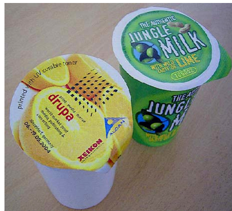
Figure 2. Dairy cups; left: printed with UV curable toner-right printed with conventional toner (no toner in sealing area)
