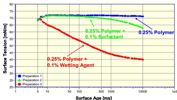
Chart 3. Dynamic surface tension of aqueous pigment preparations based on Colour Index P.Y. 155 (2% pigment content) employing different dispersant systems
