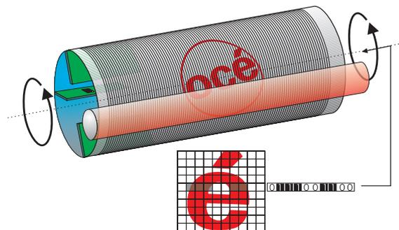
Figure 1. Direct conversion of digital data into toner-image. Schematically shown is a DI-drum with conductive tracks and a toner development roller.
