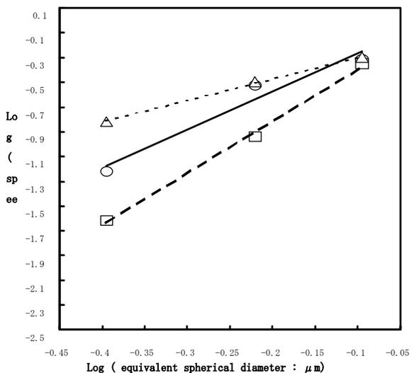
Figure 2. The relationship between the predicted speed for 80kVp X-ray irradiation and the grain size of octahedral AgBr emulsion. Circle : Unsensitized emulsion, Square : Sulfur-sensitized emulsion, Triangle : Sulfur-plus-gold-sensitized emulsion.
