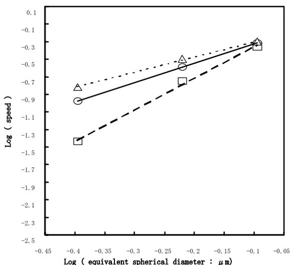
Figure 1. The relationship between the speed for 80kVp X-ray irradiation and the grain size of octahedral AgBr emulsion. Circle : Unsensitized emulsion, Square : Sulfur-sensitized emulsion, Triangle : Sulfur-plus-gold-sensitized emulsion.
