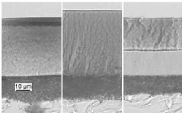
Figure 3. Location of the colorants in 3 microporous media
