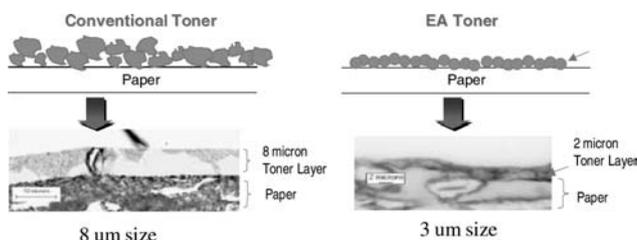
Figure 4. Thinner toner layer on substrate enabled by smaller EA toner.
