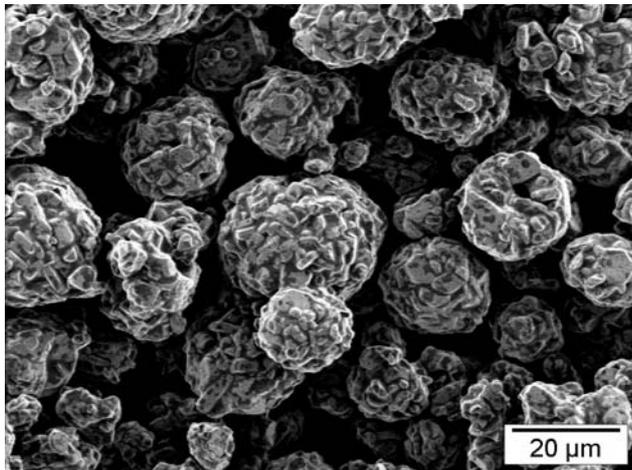
Figure 1. Scanning Electron Micrograph of small hard ferrite high definition carrier particles.
