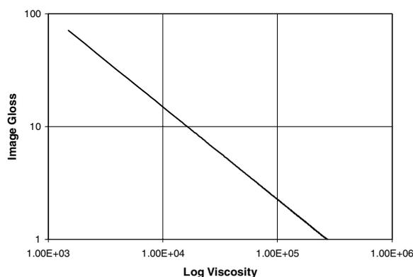
Figure 3. Dependence of Gloss on toner viscosity at constant fusing conditions.
