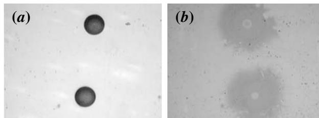
Figure 1. Optical micrographs (x100) of ink-jetted droplets on fluoro treated PET (Agfa). (a) surfactant containing jet ink (UGE 5529) with average drop diameter of 161  $\mu\text{m}$ , (b) model jet ink (U3285) without surfactant with average drop diameter of 424  $\mu\text{m}$ .
