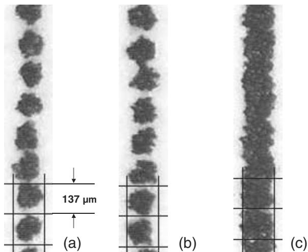
Figure 1. Lines printed onto HD125 paper in 185dpi mode with (a) single drops of 75pl, (b) single drops of 150pl, and (c) four drops of 175pl total ink volume per ink channel.
