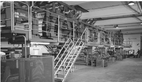
Figure 1. Conventional gravure press for laminate flooring.
