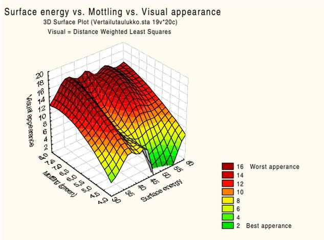
Figure 1. The effect of surface energy level on print mottle and visual quality. (The lower the mottle value, the less mottling.)
