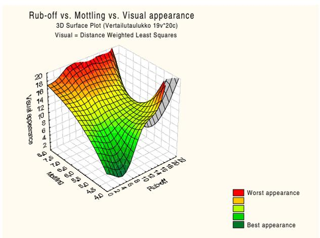
Figure 2. The effect of abrasion durability on print mottle and visual quality. (The lower the rub-off value, the better abrasion durability.)
