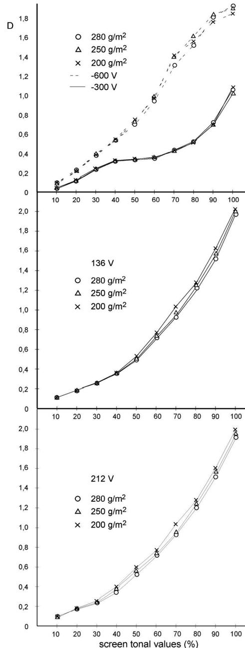
Figure 1. Inking density versus screen tonal value.
