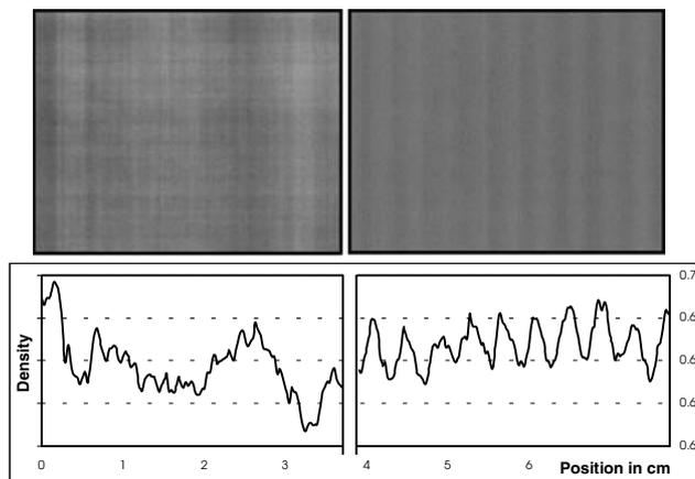
Figure 3. Streaks (left) and Banding (right) with density profiles.
