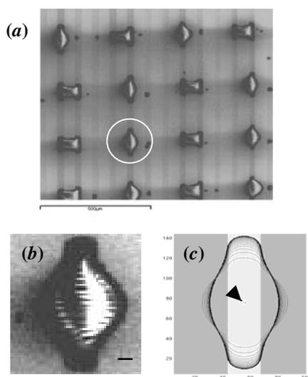
Figure 1(a): SEM image of a set of ink-jetted droplets on a chemically patterned substrate. The scale bar is 500  $\mu\text{m}$ . (b) Magnified image of the droplet circles in (a). Scale bar is 10  $\mu\text{m}$ . (c) Lattice Boltzmann simulation of droplet spreading, where the hydrophilic areas now shown by light grey. The point of impact of the droplet is indicated by an arrow.
