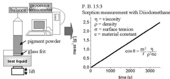
Figure 2. Measurement of surface tension for pigment powders. Owens Wendt theory provides surface polarity parameters.
