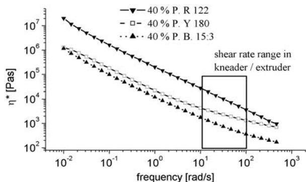
Figure 1. Rheological measurement on pigment preparations: 40 % pigment in toner resin (polyester) (at 155 °C)
