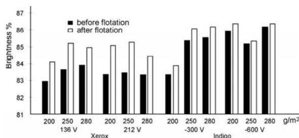
Figure 1 The effect of deinking on brightness
