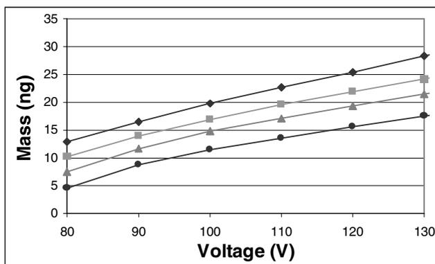
Figure 1. Change in drop mass as a function of four different nozzle diameters.
