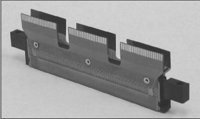
*Figure 3. SX-128 printhead with per channel connectors*
