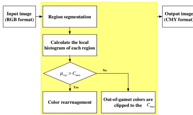
Figure 1. Block diagram of the proposed gamut mapping.
