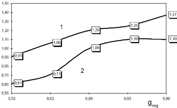
Figure 3. General gradient and gradient of the linear part of tone-reproduction curve versus development degree of negative photographic film. 1 – Gradient of a rectilinear site. 2 – General gradient of tone-reproduction curve.
