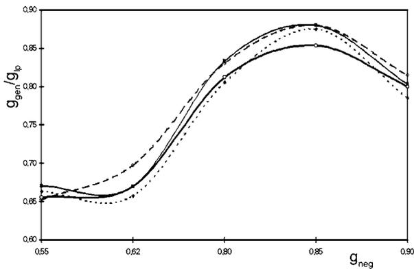
Figure 4. Relation of general gradient of the tone-reproduction curve to the gradient in half-tones versus mean gradient of negative photographic film: Nikon F4, Zenit 12, Zenit 11, Canon F1.
