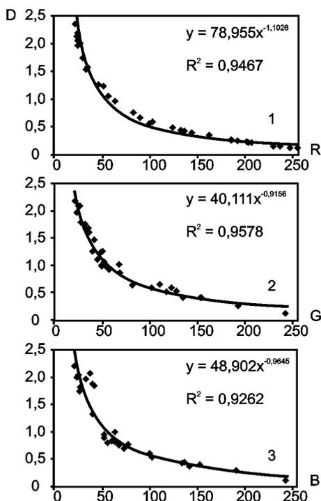
Figure 2. Calibration curves for converting RGB values into optical densities: 1-behind red filter, 2-behind green filter, 3-behind blue filter.
