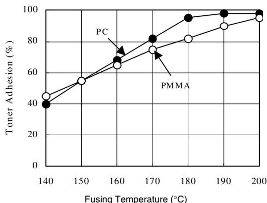
Figure 3. Toner adhesion and fusing temperature.
