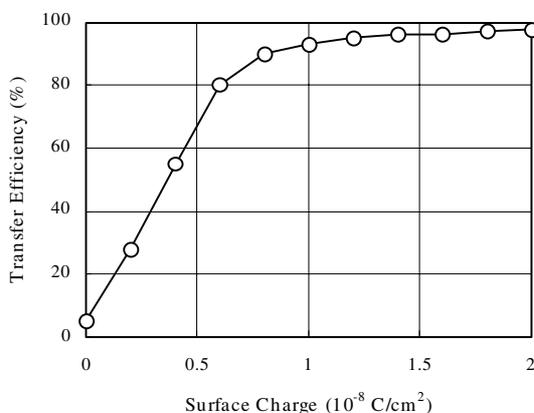
Figure 2. Transfer efficiency and surface charge.
