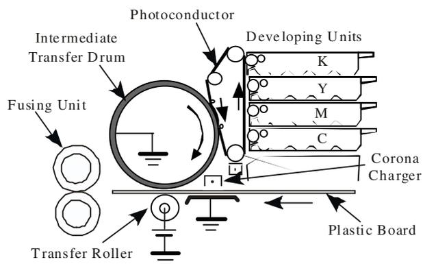
Figure 1. Construction of experimental printing machine.
