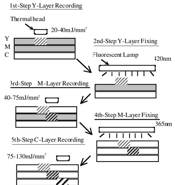
Figure 2. Full color recording process of the TA system
