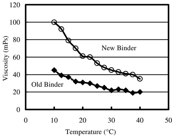
Figure 7. Relationship between viscosity and temperature of PVA solution
