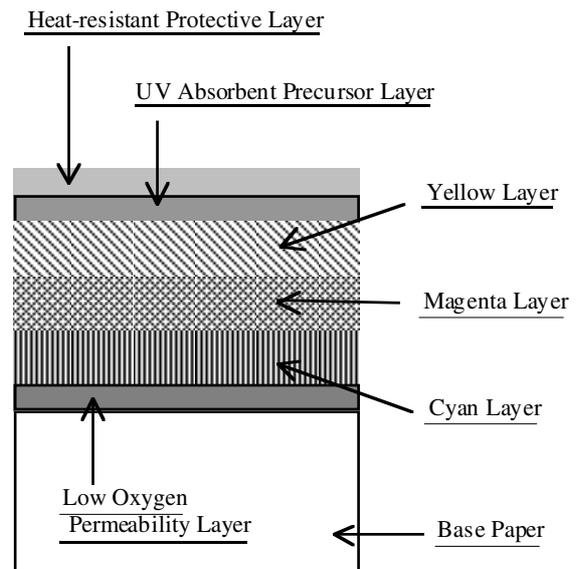
Figure 1. Simplified cross-sectional view of TA paper
