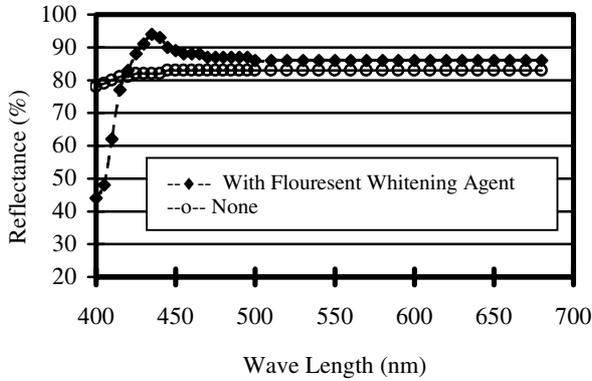
Figure 6. Effect of the fluorescent whitening agent for reflectance spectrum of TA paper
