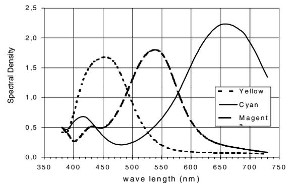
Figure 6. Spectral characteristic of photo paper
