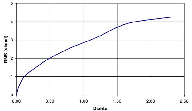
Figure 5. RMS vs. density of a laser printer on photo paper
