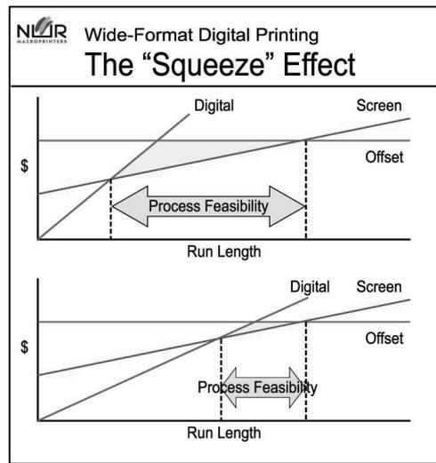
The following table describes the cut-off point between the screen-printing process and digital printing, based on the capacity of the NUR Fresco.
