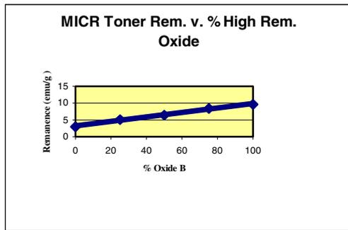
Figure 6. Variation of remanence to % oxide B
