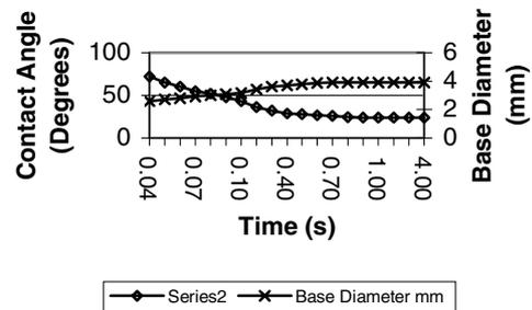
Figure 1. Change in contact angle and base diameter of ink spot on polyester label stock. Data obtained on a Fibrodatt system with a 12.5cps (at 50Deg C) UV-Curing ink
