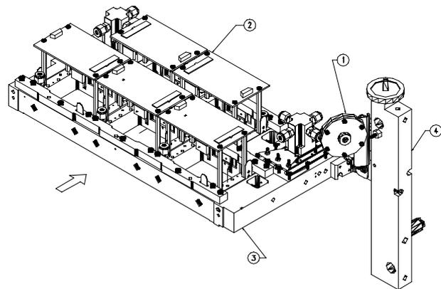
Figure 2. SP12.8/600 Single Pass Print Engine. 1: Last chance filter; 2: Five 2.56 inch print swaths; 3: Frame; 4: J-tube
