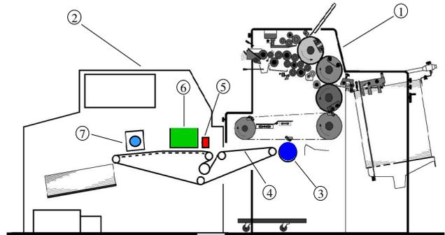
Figure 3. Combination of offset press and inkjet imprinting unit. 1: Quickmaster 46-1 offset press, 2: inkjet imprinting unit, 3: vacuum cylinder, 4: vacuum belt, 5: paper edge sensor, 6: inkjet heads, 7: UV dryer
