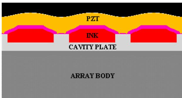
Figure 1. Spectra's shear mode technology: a cross section view of three ink pressure chambers of the 128-jet array.
