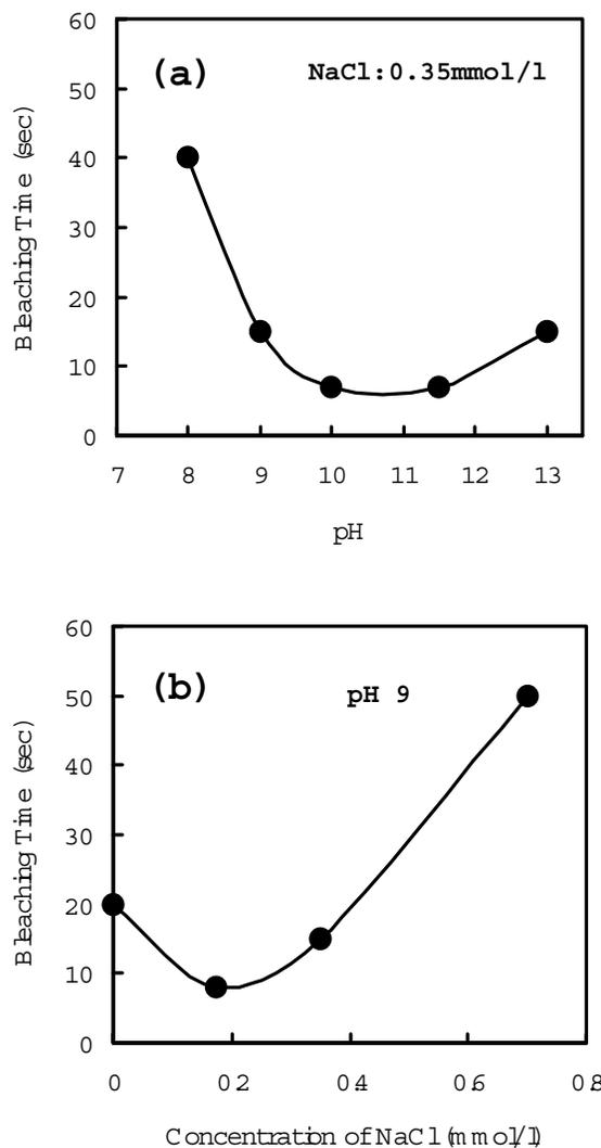
Figure 2. Effects of pH (a) and NaCl concentration (b) on bleaching speed.
