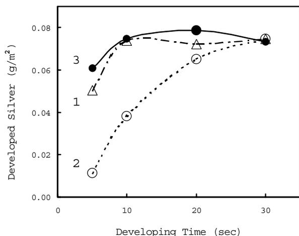
Figure 1. Effects of ascorbic acid on development speed.
