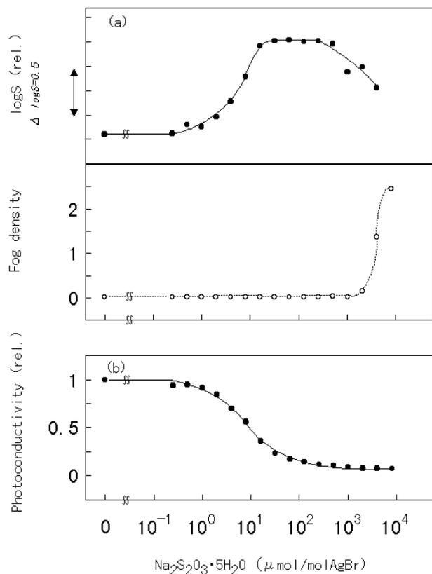
Fig.1. Photographic sensitivity  $S$  and fog density (a), and photoconductivity (b) of octahedral silver bromide grains in emulsion as a function of the amount of sodium thiosulfate used for sulfur sensitization.
