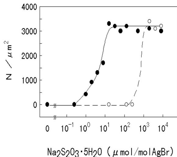
Fig.3 The number ( $N$ ) of the centers observed with (●) and without (○) the amplification treatment as a function of the amount of sodium thiosulfate.
