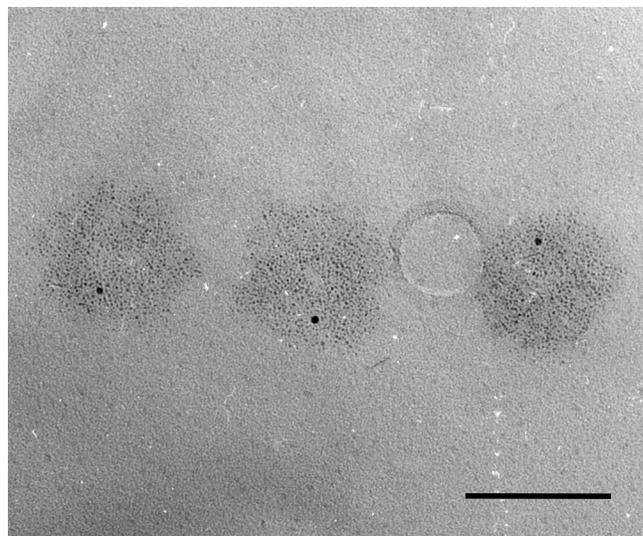
Fig.4 An electron micrograph of gelatin shells of octahedral silver bromide grains in an emulsion, which was sulfur-sensitized with sodium thiosulfate of  $16\mu\text{mol/mol}$  AgBr, being exposed for 30sec and processed with the same amplification treatment as shown in Fig.2 (b). The length of the bar in this figure refers to  $0.2\mu\text{m}$ .
