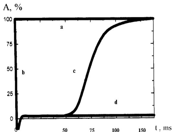
Figure 1. Kinetic curve of changing transmittance for gel under investigation a) oscilloscope signal, corresponding to 100% absorption; b) initial flash signal; c) curve of the gel; d) curve of control sample (pure glass)
