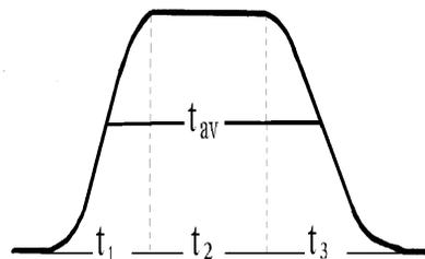
Figure 1. Quasirectangular form of electrical field impulse
