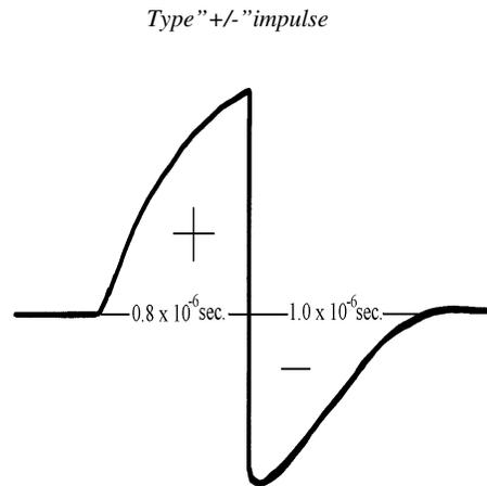
Figure 5. Altering electrical field impulse
