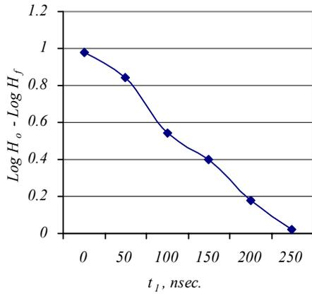
Figure 2. Effect of retention time ( $t_1$ ) on the photographic response
