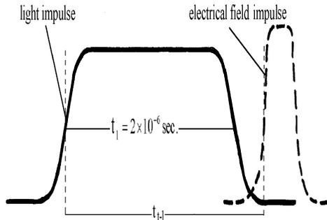
Figure 3. Sequence of light and electrical field impulse
