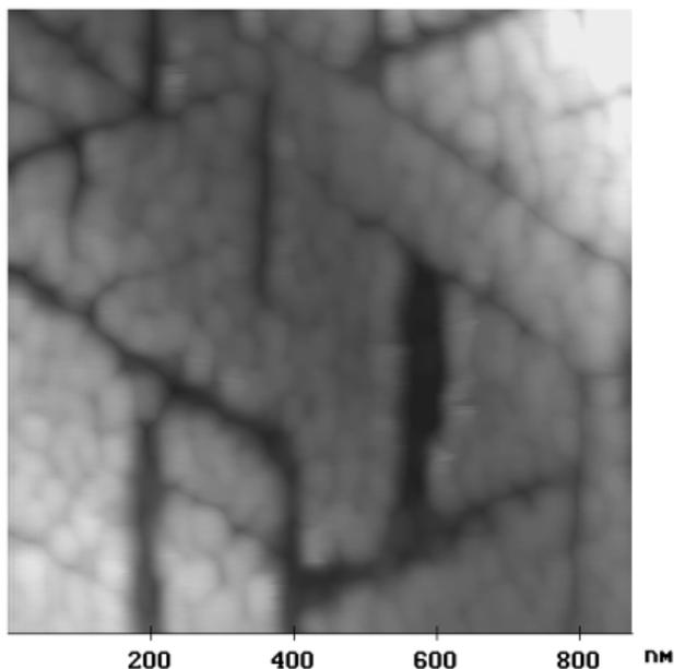
Figure 4. AFM image of Dye II rod-shaped aggregates.
