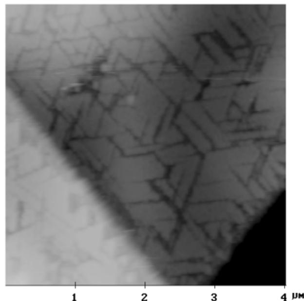
Figure 3. AFM image of two overlapping AgBr tabular grains having rod-shaped aggregates of **Dye II**.
