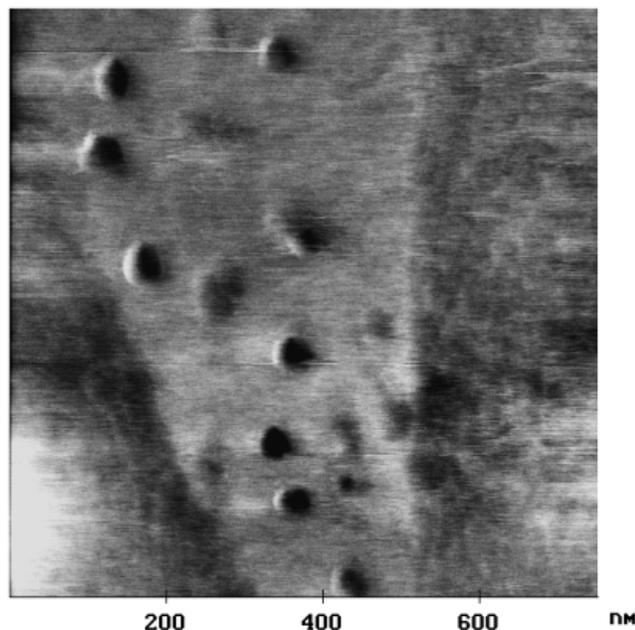
Figure 7. LFM torsional image of **Dye I** identical to Fig. 6.
