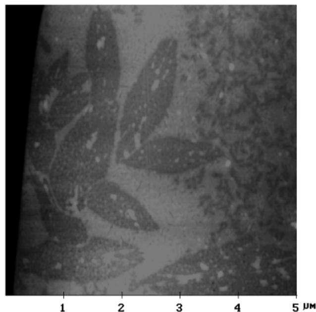
Figure 1. AFM image of **Dye I** aggregates on AgBr tabular grain.
