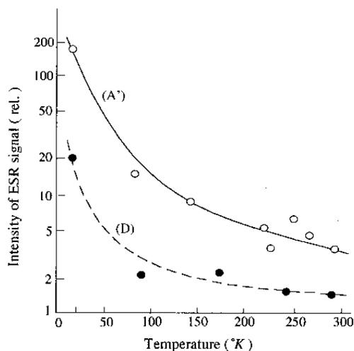
Figure 3. Temperature dependence of ESR signal intensities of clusters of Ag atoms in Samples A' and D.
