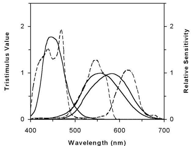
Figure 2. Color-matching function tristimulus values (solid line) compared with CNF relative spectral sensitivity (dashed line).
