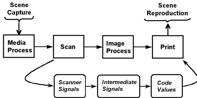
Figure 1. A basic film digitization scheme.
