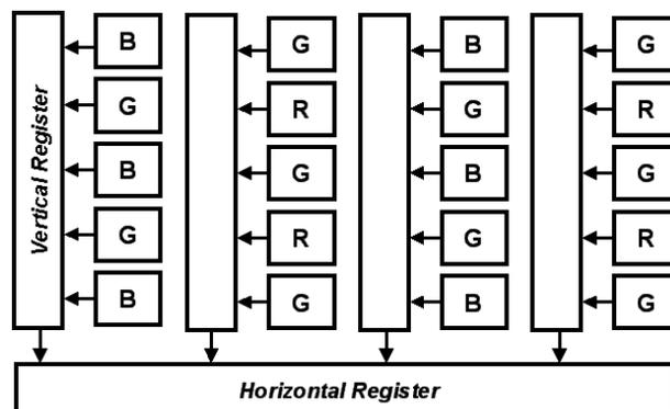
Figure 3. Segment of a typical solid state CCD capture sensor in a planar array, viewed from top-down as exposed.
