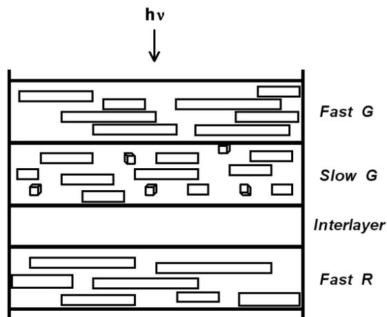
Figure 4. High-density crystal packing in a segment of a modern color negative film, as viewed in cross-section.
