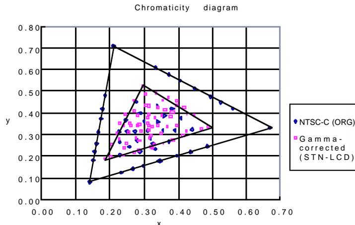
Figure 8. The gamut of gamma-corrected display values
