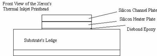
Figure 3. Front View of just the chip and substrate of Xerox's Thermal Inkjet Printhead
