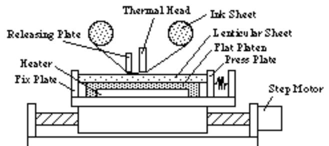
Figure 1. A schematic drawing of Motion Image Printer
