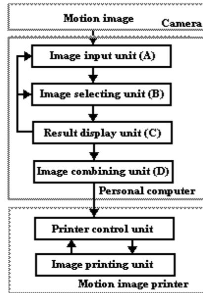
Figure 2. Construction of motion image printer system
