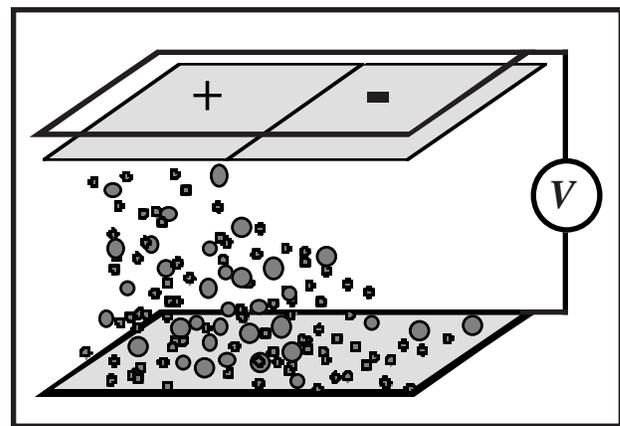
Figure 3. Schematic of a line-edge development apparatus. Toner is ejected from the lower donor surface and either attracted or repelled to areas above.
