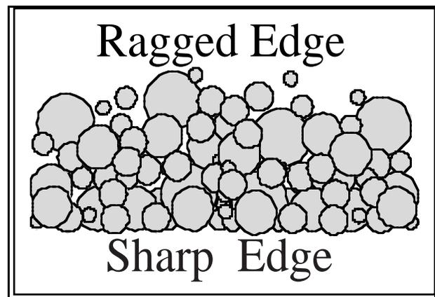
Figure 4. Particle development of a line. The top edge is drawn to illustrate poor edge quality when compared with the lower edge.
